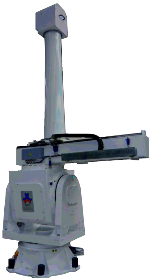
Fig. 2 : example of 5-axis positioner (P60AEA + offset table + P40R)
